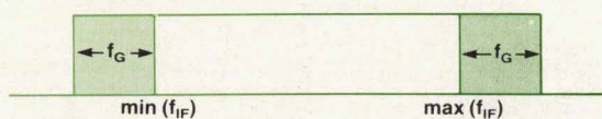
Fig. 2. IF amplifier frequency response. The guard band f_G is allocated to accommodate modulation on the input signal.
